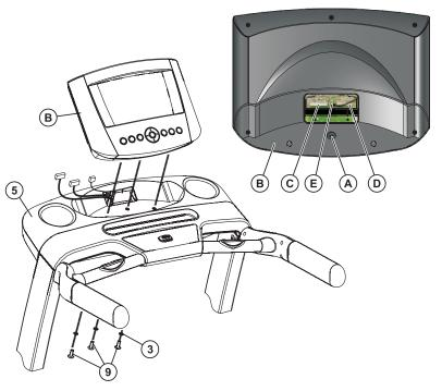
**CAUTION:** Do not pinch the wires when attaching the main console to the console bridge.
