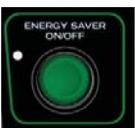
The Energy Saver Mode is used to minimize the power being pulled from the wall when the equipment is not in use. The unit will automatically go into Energy Saver Mode five minutes after ending a workout. Press the ENERGY SAVER button to either "wake up" the console or put it into the Energy Saver Mode. Energy Saver can be turned off in the Settings Menu. An indicator LED will flash while in Energy Saver Mode.
