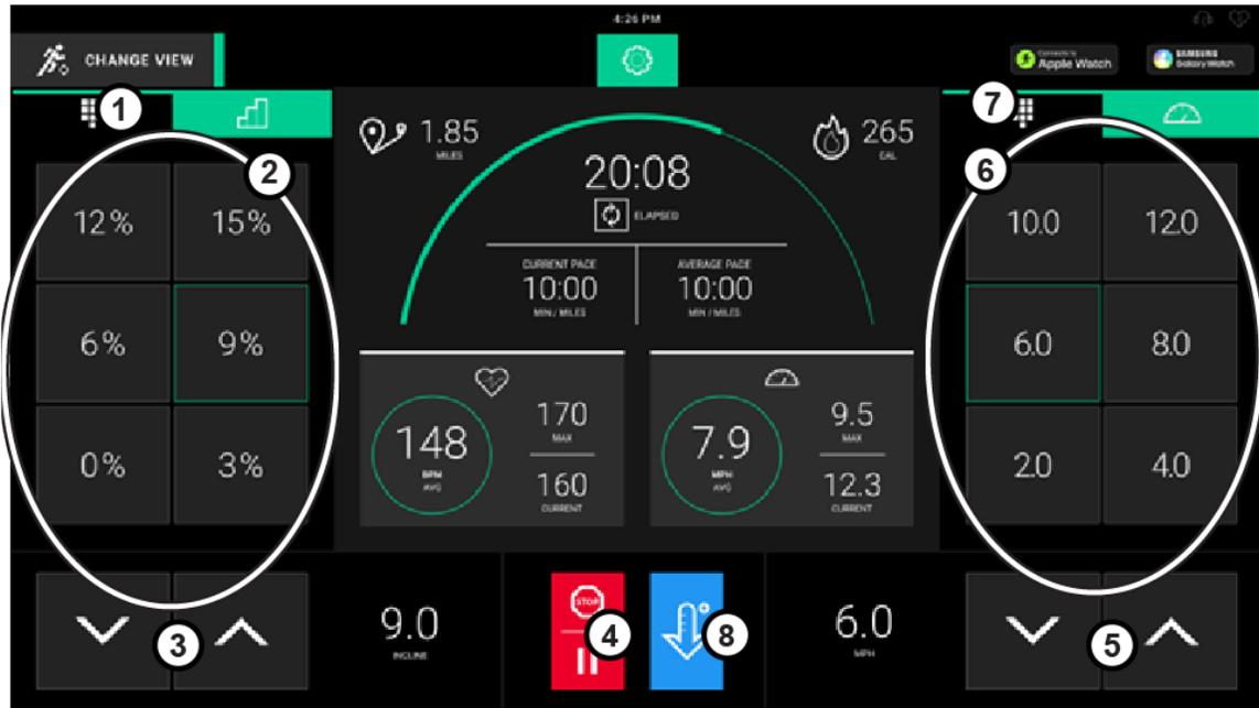
This workout is intended to help exercisers shape their own interval training by selecting the incline, speed, and time. The user defines a low speed and a high speed and can manually toggle between them via buttons.
