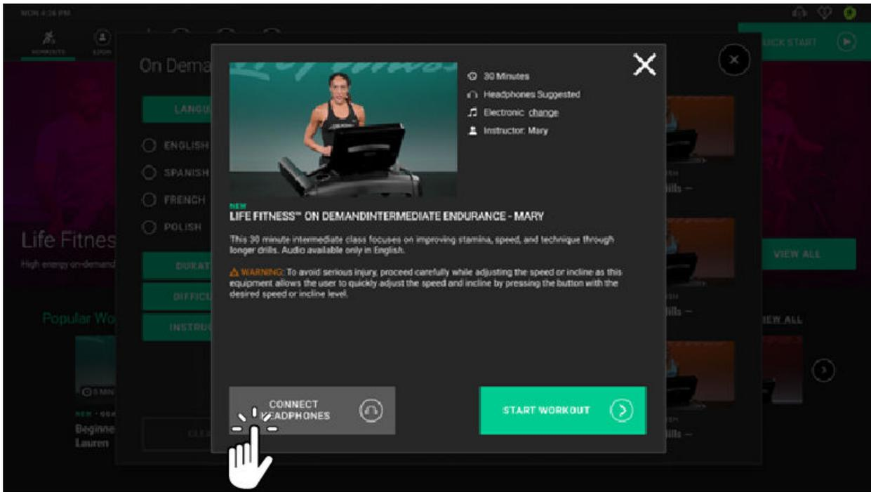
4. Use the quick-touch buttons to adjust workout settings such as speed, incline and resistance. **NOTE:** Quick-touch buttons vary depending on workout. Image shown is a treadmill workout.
