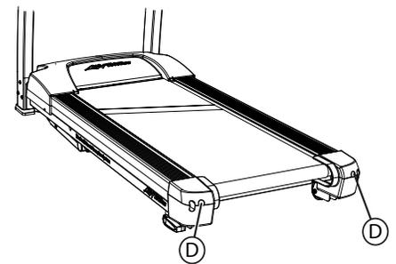
**Note:** Do not exceed one full turn of the adjusting screws in either direction. If after one full turn the belt does not track properly, contact Customer Support Services.
