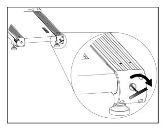
Step 3: When the belt tracking is consistent, then increase the speed to 5 mph (8 km/h) and adjust the belt if needed according to step 2.
