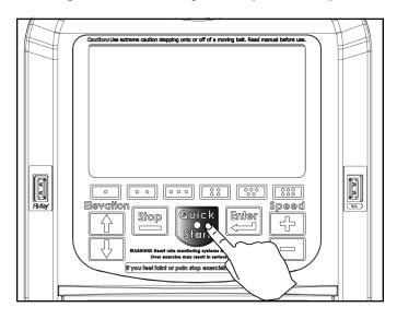
Step 2: Increase the speed to 3 mph (4.8 km/h), then grab hold of the handrails and begin to walk.
