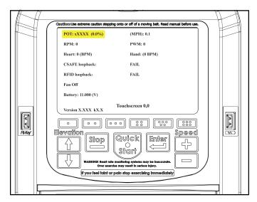
Step 3: When the calibration is complete, the "POT" category will unhighlight. You may now exit by pressing and holding the [One Dot] button, then press the [Stop] button, then release both buttons. The screen will then change to the main menu.
