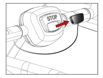
Option 2: Press the [STOP] button on the E-Stop module.
