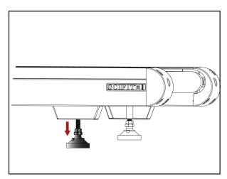
Step 4: Move the height adjustment nut back up to the top of the threads followed by the jam nut on both footpads, then tighten with the cresent wrenches.
