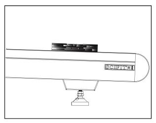
Step 2: Use the cresent wrenches to loosen the height adjustment nut (item 1) and jam nut (item 2) on both right and left footpads.
