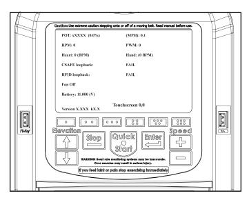
Step 2: Standing off of the machine press the elevation [Up Arrow] and [Down Arrow] buttons at the same time, this will highlight the "POT" category yellow and the calibration process will begin.
