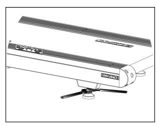
Step 3: Lift and stabilize the rear of the treadmill until the machine is level (see bubble on the level), then adjust the right and left footpads until they touch the floor.
