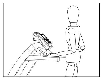
Step 3: Stomp your foot in front of the motor cover. If the belt slips return to the "Belt Alignment/Tension" section.
